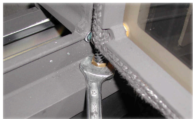
Im. 1: Turning the brass nut
